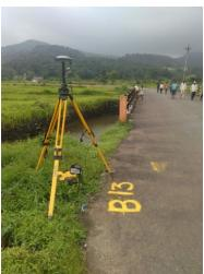
There are two DGPS Control points i.e., Control point and Land survey. Control points are carried out to establish networks of points and these points are used for measurements. Hence, these site points are recorded for highest precision.
